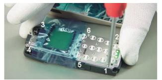
Remove the six screws with screwdriver Torx T6 in Before removing the UI module LU9 this clip has the shown order. When assembling the reverse order has to be taken with a torque of 17Ncm.
