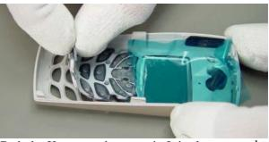
Grab the Keymatand remove it. It is always good to protect the window also from the inner side.
