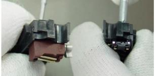
The System Connector contains Vibra Motor and Microphone, which can be easily pushed out of the System Connector.
