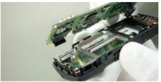
Lift up the CMT module LA5 carefully. Sometimesit happens that the battery connector gets stuck at the SIM Card Cover. Take care not to bend the spring contacts of the battery connector.
